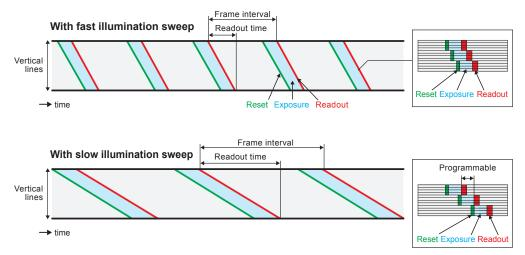
Engineered with high speed, large field of view experiments in mind, the ORCA-Lightning employs a unique readout method allowing it to achieve unmatched frame rates. By concurrently reading four lines at a time, image data is streamed at up to 121 full frames (4608 x 2592) per second using Hamamatsu's patented Lightsheet Readout Mode.
